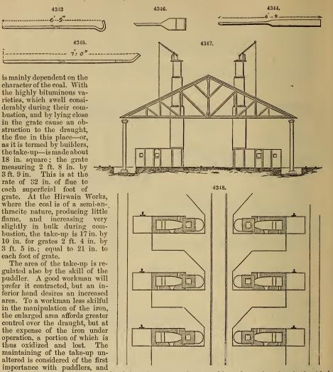
where it is constructed with fire-brick its enlargement after a week's work requires that it should be taken down and renewed. Sandstone, from its greater durability, has been adopted at some works. If the take-up be not reconstructed of the original size, the yield of metal becomes worse as the area is enlarged. Hence, with a forge of good workmen, we find that as the time approaches for repairing the yield of iron a ton is augmented.
